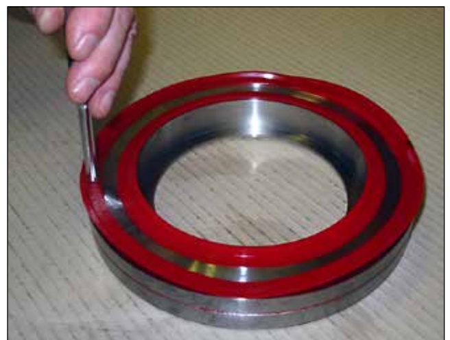
Using a blunt nose tool push the seal fully into the seal clip housing, work around the periphery of the seal until the seal is completely inserted into the clip housing
