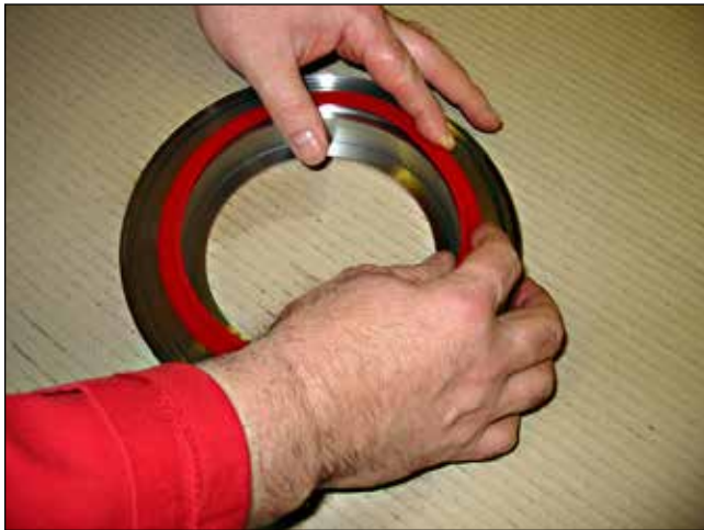
Insert the inner seal into the seal housing, the seal clip fits into the seal clip housing
