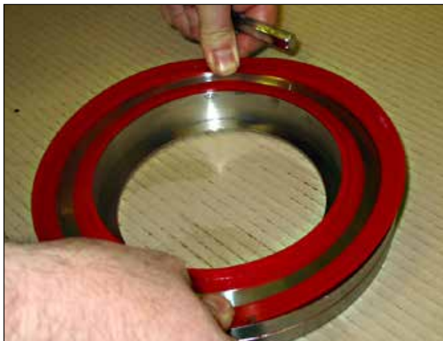
Insert the outer seal into the seal housing, the seal clip fits into the seal clip housing.
