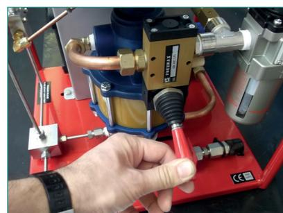
Safety On/Off Valve - Handle held down = On
