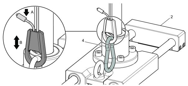
3. Lift the horizontal unit (2) until the balancer (5) can be inserted into the upright shaft (3).
